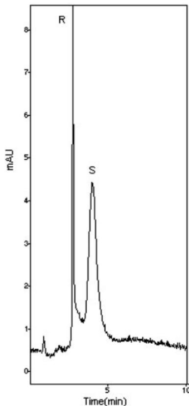
**Figure 6.** Chiral separation of an ibuprofen sample enriched in the *S*-form (enantiomeric purity *R*:*S* = 1:6). Experiment was performed at 15 kV. The sample was injected electrokinetically at 1 kV for 3 s. The capillary was thermostated to 25°C. Detection wavelength was set at 254 nm. The electrolyte used was composed of ACN-phosphate buffer (pH 3.2, 20 mM) (50:50 v/v).
