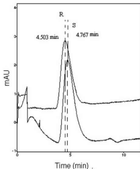
**Figure 1.** Chiral recognition of racemic ibuprofen on MIP1 (100  $\mu\text{m}$  id  $\times$  20 cm) at 15 kV. The sample was injected electrokinetically at 1 kV for 3 s. The capillary was thermostated to 25°C. Detection wavelength was set at 254 nm. The electrolyte used was composed of ACN-phosphate buffer (pH 3.2, 20 mM) (50:50 v/v).
