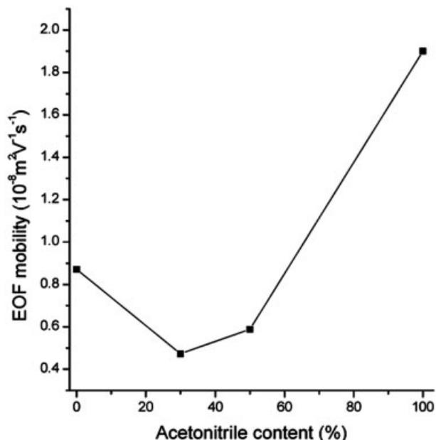
**Figure 4.** Effect of ACN content on the EOF mobility on MIP4 in nonaqueous mode. Experimental conditions: mobile phase, ACN/methanol (v/v) in different ratios in 1% acetic acid; applied voltage, 20 kV.
