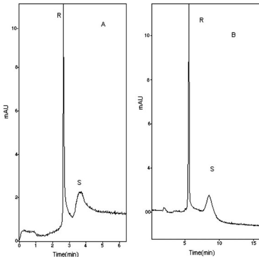
**Figure 5.** Chiral recognition of racemic ibuprofen on MIP4 (A) and MIP5 (B) at 15 kV. The sample was injected electrokinetically at 1 kV for 3 s. The capillary was thermostated to 25°C. Detection wavelength was set at 254 nm. The electrolyte used was composed of ACN-phosphate buffer (pH 3.2, 20 mM) (50:50 v/v).
