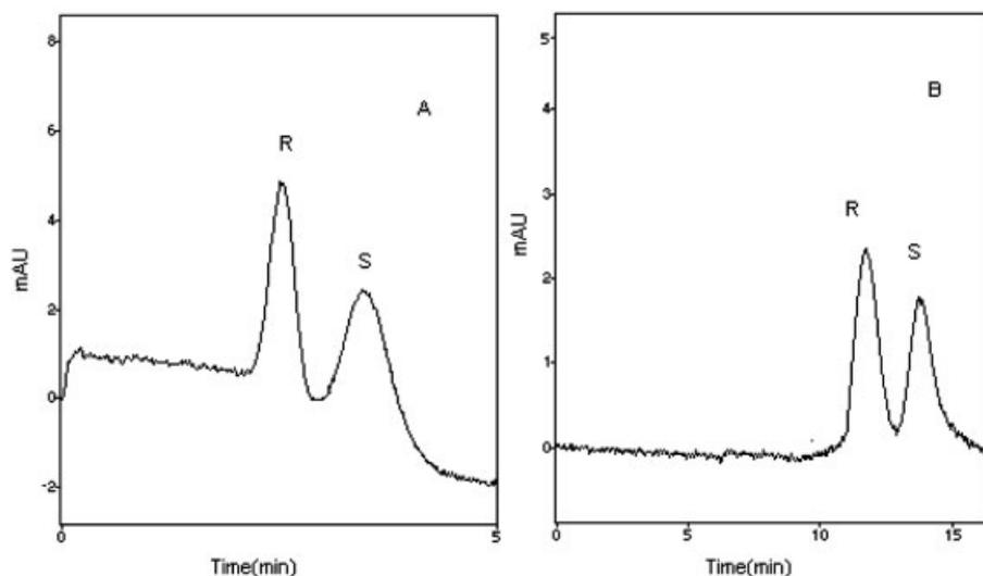
**Figure 7.** Chiral recognition of racemic ibuprofen on MIP4 at 20 kV. The electrolyte used was composed of methanol/acetic acid (99:1 v/v) (A) and 1% acetic acid in methanol/ACN (70/30 v/v) (B). The sample was injected electrokinetically at 1 kV for 3 s. The capillary was thermostated to 25°C. Detection wavelength was set at 254 nm.
